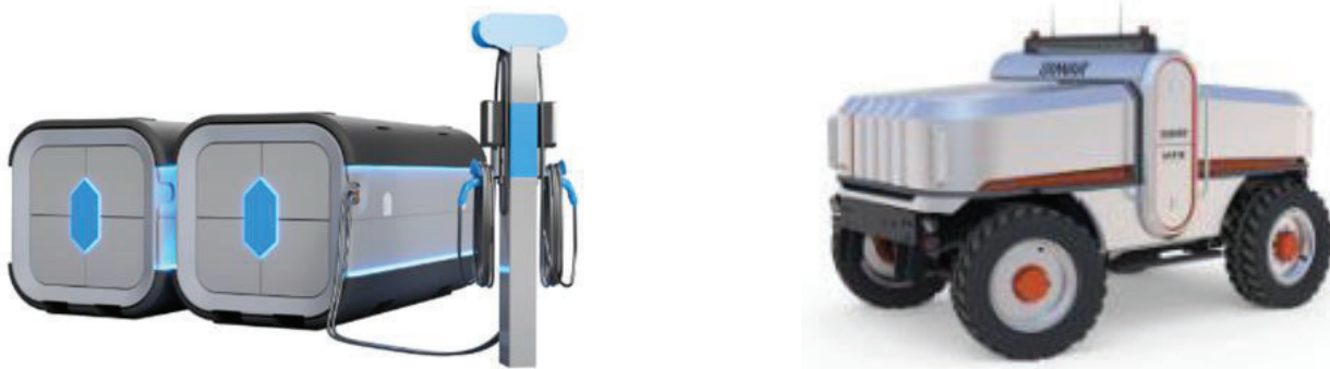
FIGURE 8: JOULE'S MODULAR, STACKABLE, CHAINABLE BATTERY SYSTEM (LEFT), DANNAR MOBILE POWER STATION (RIGHT)
